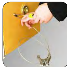
Anti-Static Device: conductor grip combine the equipment with the cabinet to conduct the static to earth, thus to prevent
